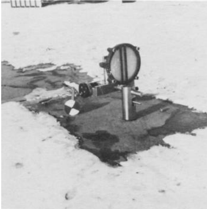
Figure 6-5. Inserted Micrometer Alignment Target. (Photo by WES)
