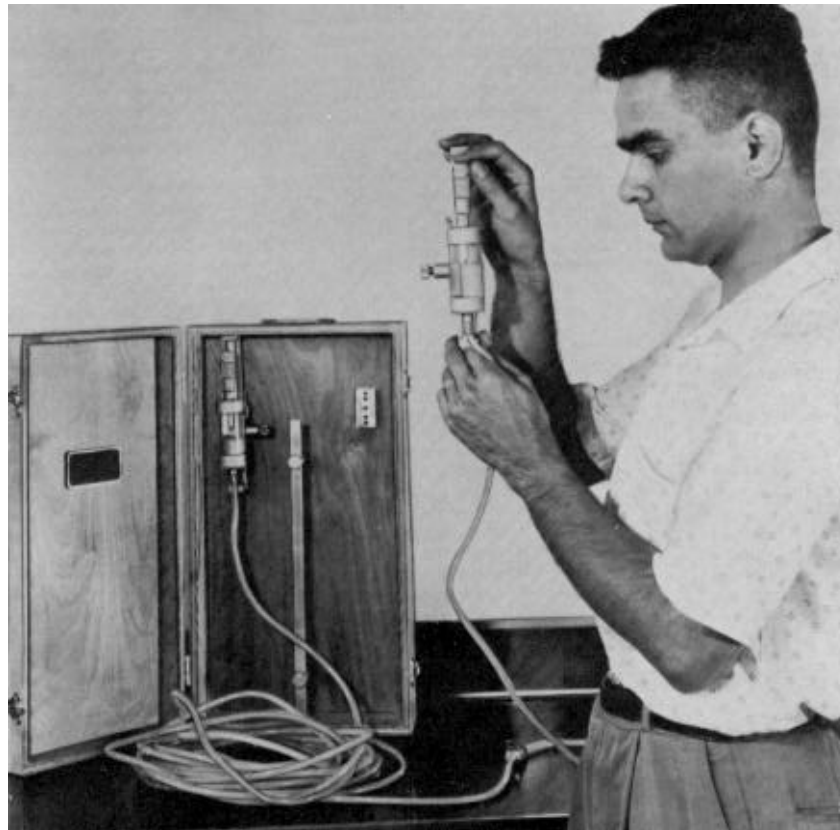
Figure 4-20. Autocollimating Tilt Measurement System
